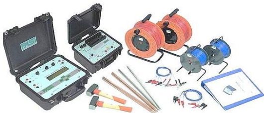
Fig. 4 Basic field equipment for this research, Pasi Terrameter, Metal Electrodes, Cables, Cutlass, Hammer, Compass and clips.
