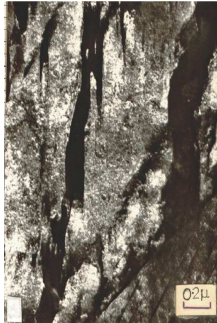
Plate 1: HRDF showing typical martensite laths. The ample was reduced 20% by rolling at -196^\circ\text{C} .
