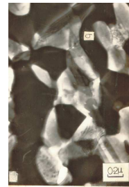
Plate 2: Bright field (BF) illustrates the occurrence of \sigma in the ferritic alloy. Alloy was deformed 80% at -196^\circ\text{C} and annealed at 700^\circ\text{C} .
