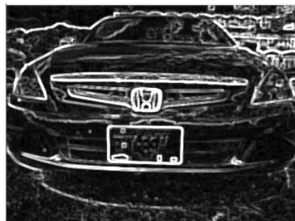
Figure 9: Result of image dilation after the Sobel edge detection.
