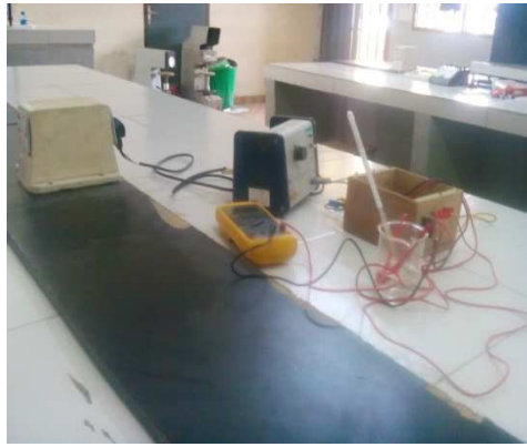
Figure 2: Picture showing the experimental set-up for the laboratory measurement of sample conductivity
