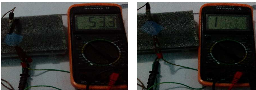
Fig 2: continuity test of conductive and non-conductive side of ITO glass slides
