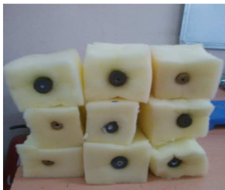
Fig. 2: Insulated metal rod samples in Styrofoam cylinder
