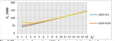
Fig. 9 Illustration of equation (19) showing variation of total system cost with storage capacity.
