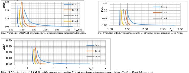
Fig. 5 Variation of LOLP with array capacity  $C_A$  at various storage capacities  $C_S$  for Port Harcourt. Iso-reliability lines for LOLP = 0.1, 0.05, 0.01 and 0.001 were obtained for each location from figures 3, 4 and 5 as follows:
