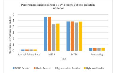
Figure 5: Performance Indices of Four 11 kV Feeders of Ugbowo 2x15 MVA, 33/11 kV Distribution Network.
