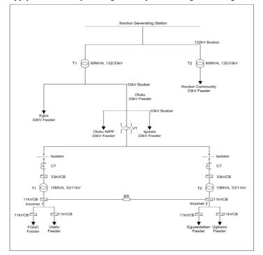
Figure 1: Single Line Diagram (SLD) of the Ugbowo 2x15 MVA, 33/11 kV Distribution Network feeders and the 132/33 kV Supply from Ihovbor Generating Station.
